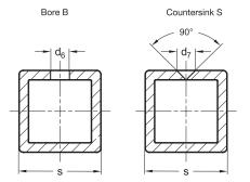
The square dimensions of the locking slide units are designed for construction tubes GN 990. These can be fitted with locking holes (B or S) by the user according to the dimensions specified in the table. Construction tubes with locking holes can be ordered as standard part GN 990.1. (see page ) cut to length and completely ready for
